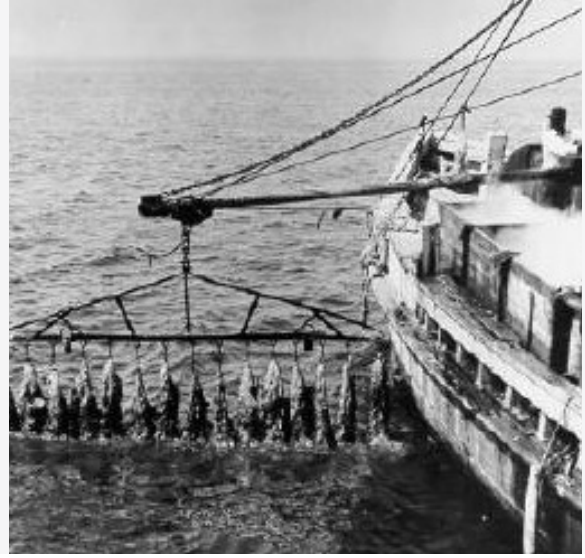
Figure 9b: Starfish mop used to control predation on shellfish beds. NOAA Fisheries Service
