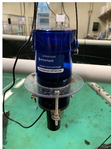
Figure 6.1: Vibratory feeder Juvenile lumpfish tank at the UNH Coastal Marine Laboratory with feed supplied via a vibratory autofeeder.
