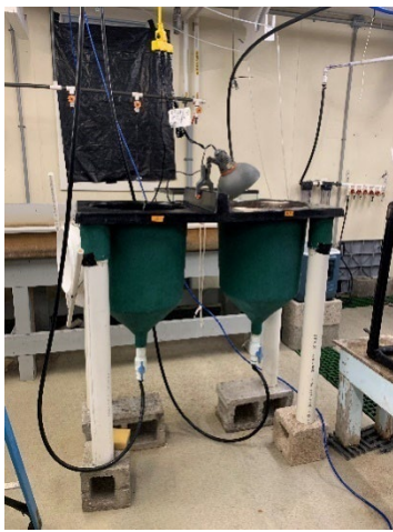
Figure 4.3: Artemia enrichment tank set up
